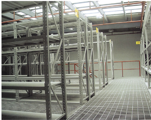
(实景) 日产汽车配送中心,使用大昌楼阁式货架. Dachang mezzanine storage built in Nissan motor's 4S shop.
