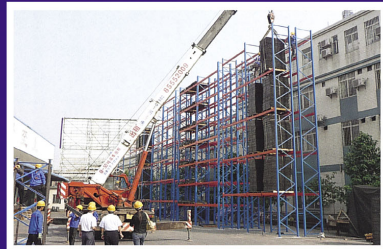
高层重型货架经严格载重测试,重量每层达5吨 The heavy duty shelves are subjected to a rigorous load test with a weight of 5 tons per floor
