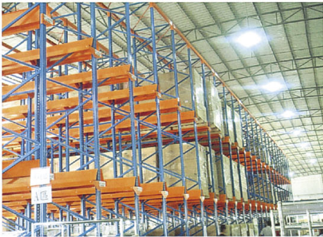
DC-90通廊式仓库货架 DC-90 Drive-in/Drive-through Racks
