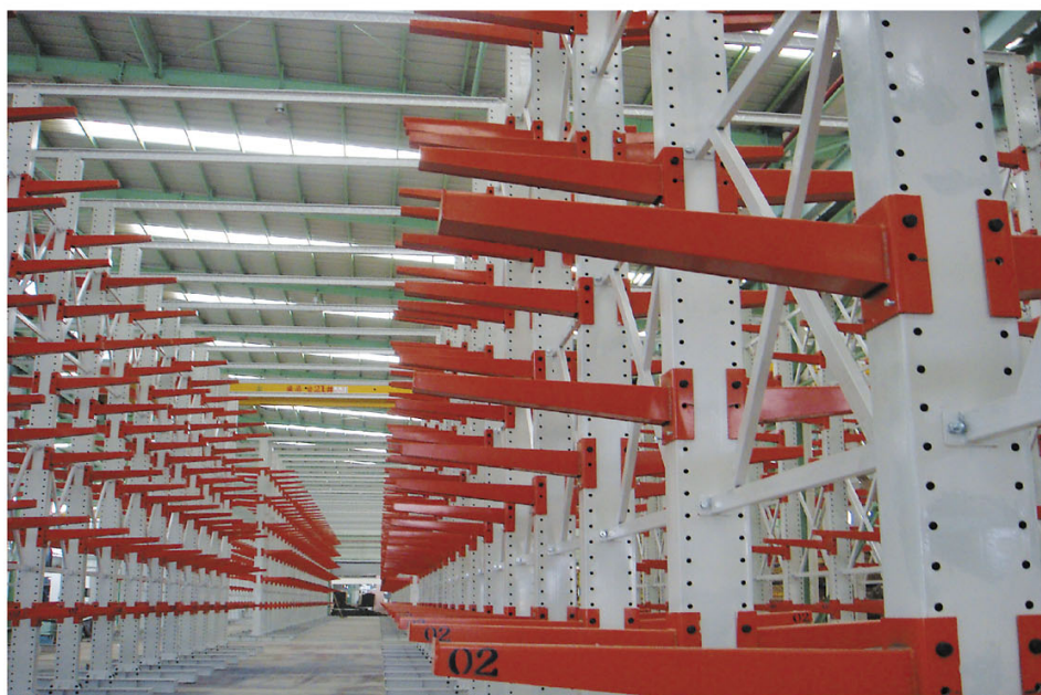
坚美铝业安装实景图 Cantilever storage system in JianMei Aluminium
