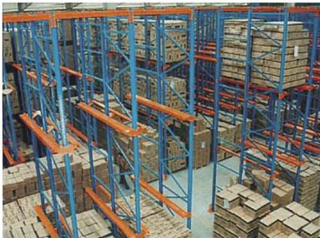
DC-90通廊式仓库货架 DC-90 Drive-in/Drive-through Racks
