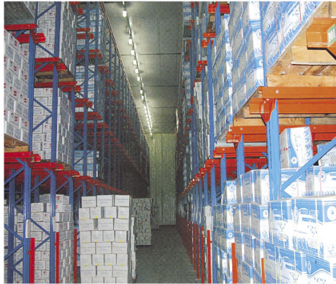
通廊式仓库货架导轨 Roll formed pallet rail
